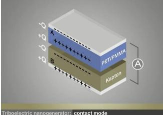
**Figure 1. Triboelectric Generator**
